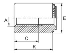
Female thread A = M4Height K = 10Min distance to edge = 4.0Outer diameter E = 8Plate thickness = 1.5 to 2.3
